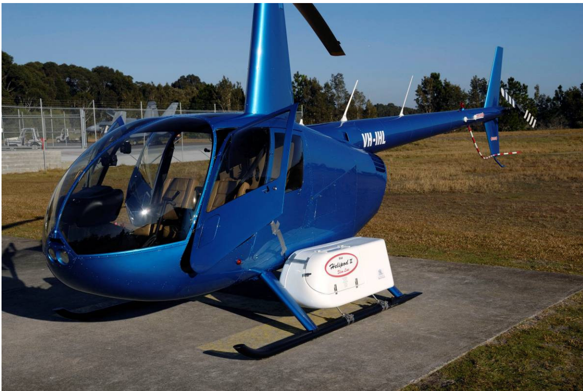
Figure 1. Helicopter with helipod (containing SFAPS system)
