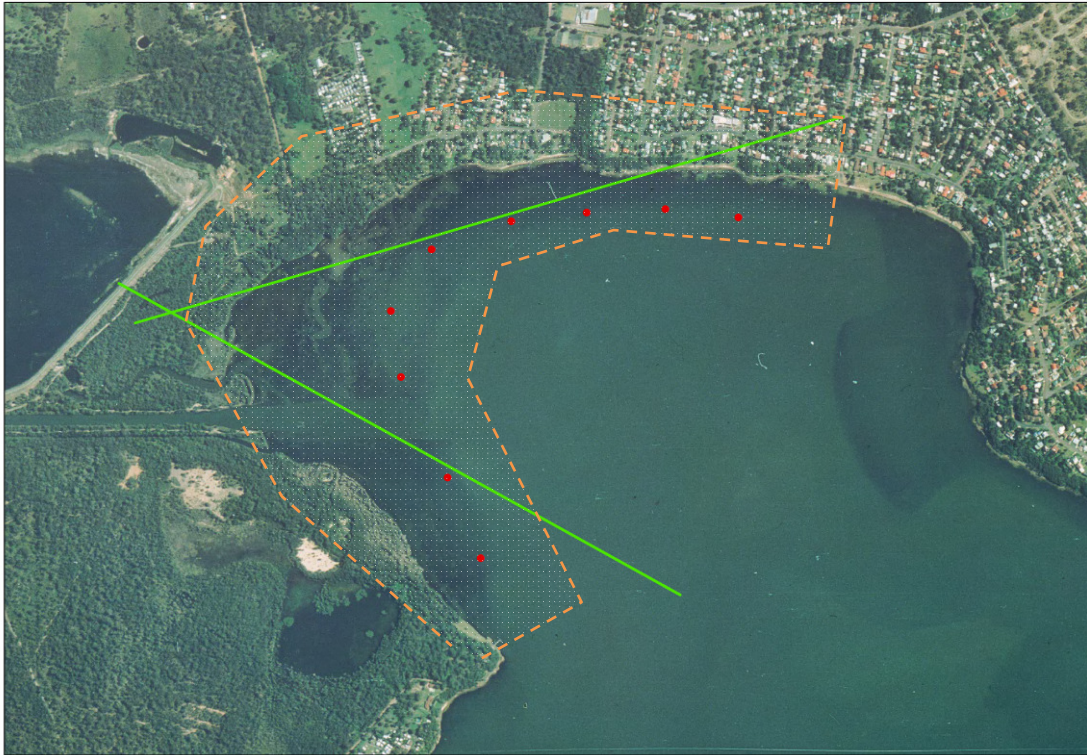
Figure 2. The area of Lake Munmorah covered in the case study (orange boundary). The green lines indicate the flight lines and the red points the floating ground control markers. Image courtesy of LMPA.
