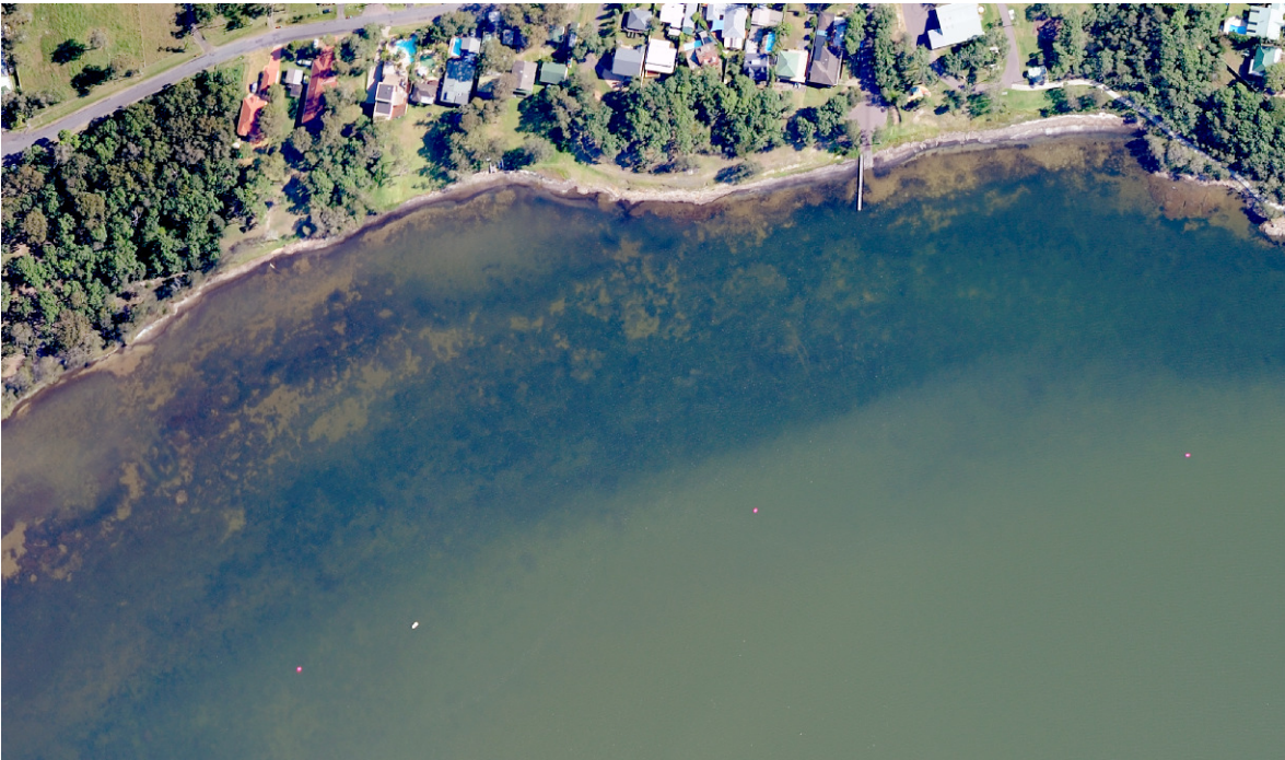
Figure 5. A higher resolution image showing the detail captured using this SFAPS. Considerable detail can be discerned in the seagrass beds. The pink floating GCP markers are also visible in the lower half of the image.
